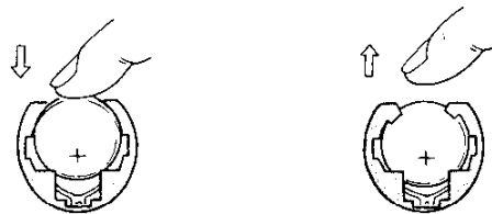
Slide battery inward, then pry up to eject
